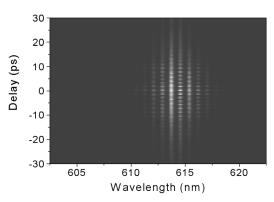
Fig. 3. SHG FROG trace of the multiwavelength Cr:forsterite laser output when the cover glass is inserted normally to the laser beam.
