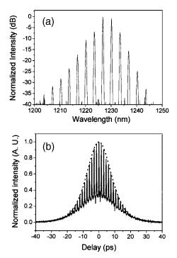
Fig. 2. (a) Output spectrum and (b) its corresponding autocorrelation trace of the multiwavelength Cr:forsterite laser output when the cover glass is inserted normally to the laser beam. The dotted curve in (b) is a sech<sup>2</sup> fitting.
