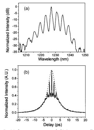
Fig. 5. (a) Output spectrum and (b) its corresponding autocorrelation trace of the multiwavelength Cr:forsterite laser output when the cover glass is turned  $50^{\circ}$  from normal incidence. The dotted curve in (b) is a Lorenzian fit.
