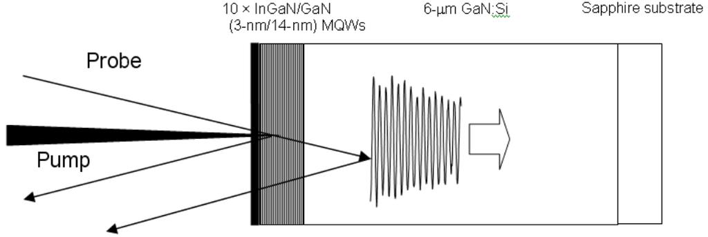
FIG. 1: Sample structures of the GaN MQW sample. Nano-acoustic waves can be generated by the pump of blue femtosecond pulses. The phonon lifetime can then be monitored by the probe pulse with Fabry-Perot type interference.
