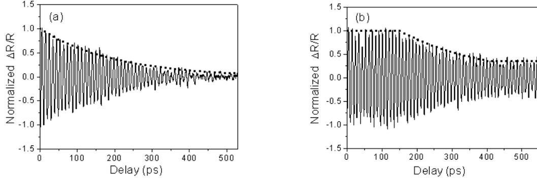
FIG. 2: The measured changes in differential reflection as a function of time delay (a) for heteroepitaxial growth and (b) in the region of lateral growth. The dotted curve in (a) is the curve used for fitting the lifetime of nano-acoustic waves, and it shows a 200-ps exponential decay.
